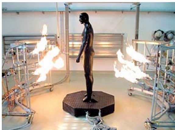
Application to test the heat-resistance of clothing: Thermo-man : Fast thermocouples places on the outside of the special dummy. Digital I/O to check and control the state of the valves of the burners.
