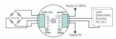
Note: The OV (supply) is internally connected to the OV (signal)
